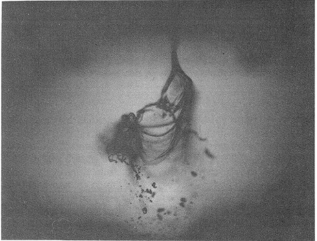
Fig. 5 "Stretched streamwise ligament breakup" (Stapper and Samuelsen, 1990): water sheet at 1 m/s with 20 m/s co-flow air: (a) face view, (b) side view
